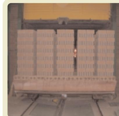
LA BOCCA DI INGRESSO DI UN FORNO A TUNNEL
